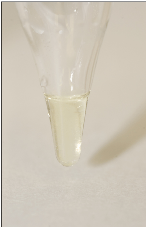
Photo 4 - Faint Yellow Color from Addition of Conc. HCl to the Reddish Solution (i.e., from Diazepam)
